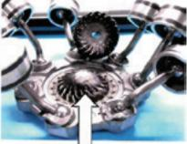
Centre Ball has melted and welded it's self to the fixed gear due to insufficient cooling through loss of refrigerant and/or
